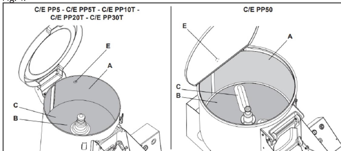
LORS DU REMPLISSAGE DU RÉCIPENT AVEC LE PRODUIT À ÉPLUCHER, NOUS RECOMMANDONS UNE HAUTEUR DE REMPLISSAGE MAXIMALE D'ENVIRON 7 CM À PARTIR DU BORD DU RÉCIPENT. CE N'EST QU'AINSI QUE LE PRODUIT AURA UNE LIBERTÉ DE MOUVEMENT SUFFISANTE PENDANT LA PHASE DE TRAITEMENT.
